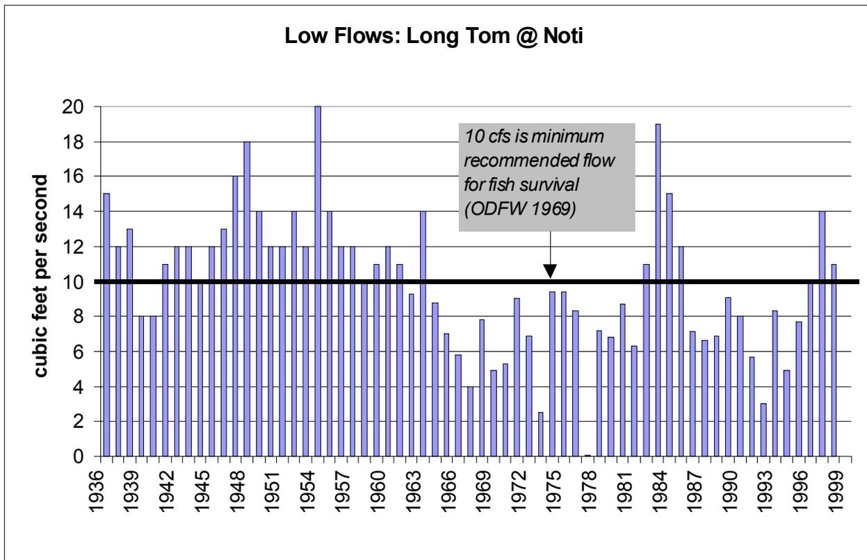
**Figure 5.2. Low flows in the Long Tom River, measured at Noti.** For each water year (Oct. 1 of previous year through Sept. 30 of labeled year), the lowest daily flow is shown (Data from USGS). The darker line at 10 cfs shows the minimum recommended flow for the months in which low flow occurred. One exception: in 1976 the low flow was in July and minimum rec. flow then is 15 cfs (Data from ODFW).
