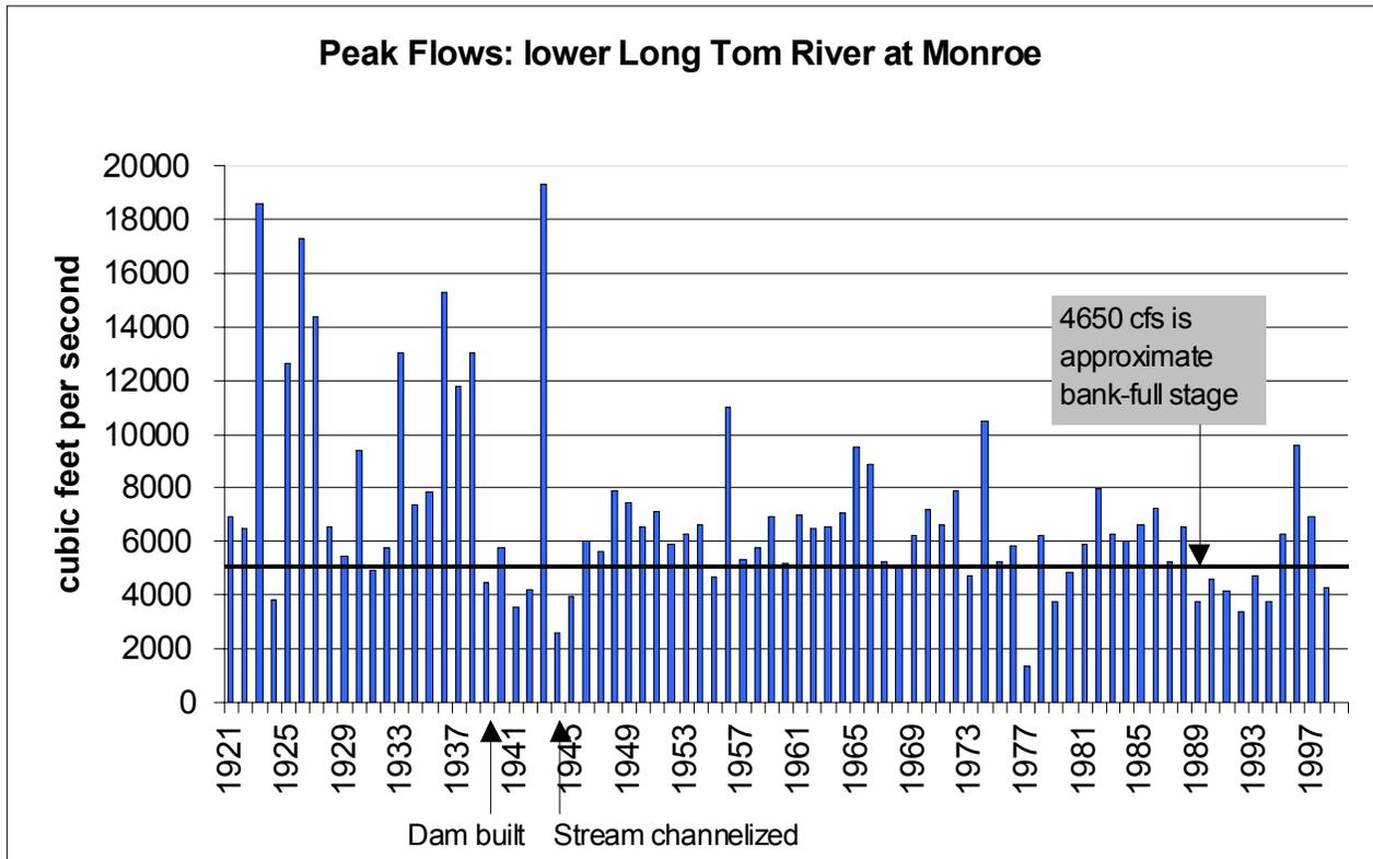
**Figure 5.1. Peak flow history of the lower Long Tom River, measured at Monroe.** Notice that after the dam was built in 1939-1941 there was a peak flow that we know from aerial photography reached flood stage. The newly built dam could not hold all the floodwaters. This prompted channelization of the 23.5 miles of lower Long Tom River below the dam during 1943-1951. The combined projects have significantly reduced peak flows since then.
